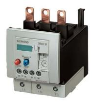
Overload relay 36...50 A For motor protection Size S3, Class 10 Contactor mounting Main circuit: Screw terminal Auxiliary circuit: Screw terminal Manual-Automatic-Reset !!! Phased-out product !!! Successor is SIRIUS 3RU2 Preferred successor type is >>3RU2136-4GB0<<
